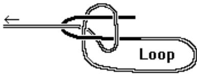
**Bowline** —used to make a loop in the end of the cord. To tie: "the rabbit runs up the hole, around the tree, and back down the hole." Essentially the same knot as the sheet bend but used to make a loop.
